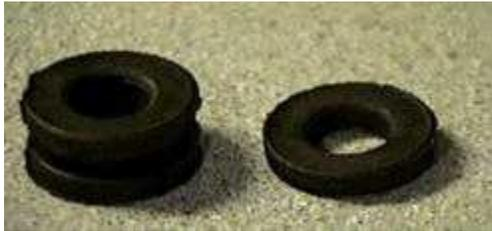
After you've gotten the handle off of the shaft completely, take one of those rubber grommets and cut in half width-wise. **Update:** Since first doing this mod, I've now decided that everyone would be better off using a washer (nylon preferably) instead of cutting a stock grommet. The first reason is that now you can always return your car back to stock. The second reason is that the black rubber on the grommet will rub off after a while and gum up the nylon bushing and shaft.
