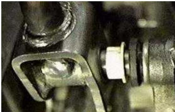
Slide one half of the grommet over the shaft [nylon&grommet].
