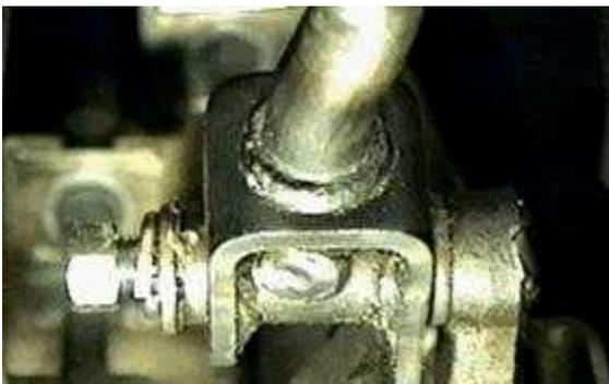
Remove the 14mm nut from the main shifter rod. Slide the shifter rod off to the driver's side (much harder than it sounds, you might have to push the plastic of the console back) and keep the 2 washers and the 2 white nylon bushings. **Update:** You can save yourself about 10 minutes by undoing that shifter link first (removing the cotter pin and detaching the link).
