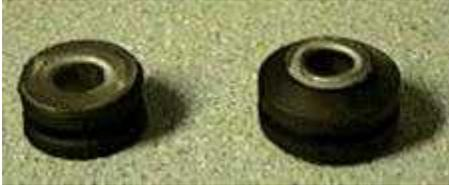
This mod has been successfully performed on a 90-94 GSX - but you don't have to have a turbo or AWD to perform this mod. There are some slight differences in bushing/grommet sizes, picture shows smaller bushing and hole diameter of the 90 on the left, and the larger grommet/bushing design of the 91-92 on the right.
