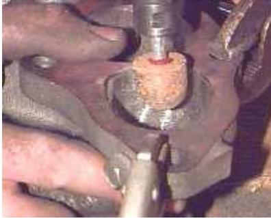
Here I am grinding away after using the carbide burr to shape it. That extra curvature around the turbine chamber should help control boost creep, as the flow out of the wastegate hole will be obstructed less. Do I have proof? Sorta.
