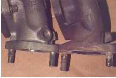
Closeup of the lower flange on a 2G (left) and 1G O2 housing. If you look at them side-by-side, you can see that the 2G wastegate runner is larger than the 1G by a little bit. It also connects back to the turbine runner at a slightly different angle.
