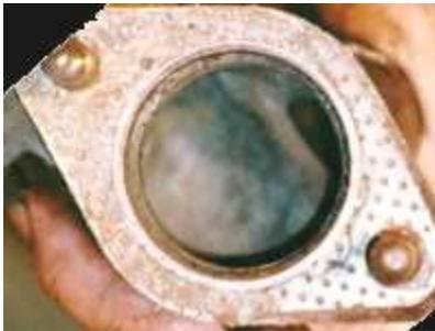
This is a look at the stock 1G O2 housing. I ground down the divider you see in it, and enlarged the outlet a good bit to match it to the stock gasket.
