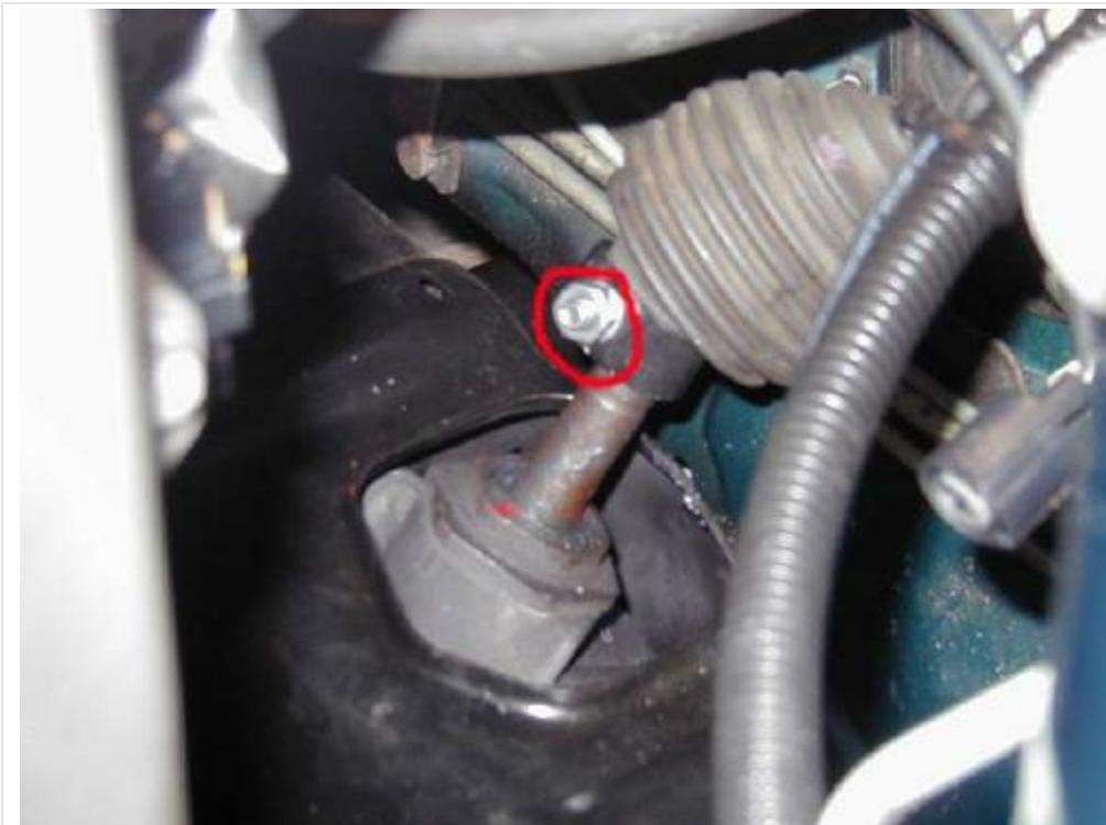
11. Now is time to remove the rack. The rack is held on by 2 brackets each using 2 17mm bolts, remove the bolts and the rack is ready to drop. It isn't that heavy, but if the rubber mounts aren't stuck to the body, then it will drop quick.
