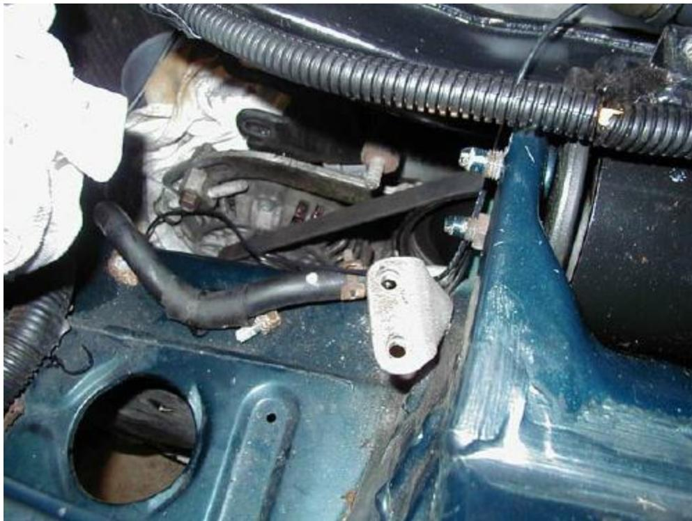
4. I removed the power steering cooling lines next, they are held on by 1 bolt that bolts into a vertical cross member behind the bumper. Assuming you don't have a FMIC they will be visible from the front.
